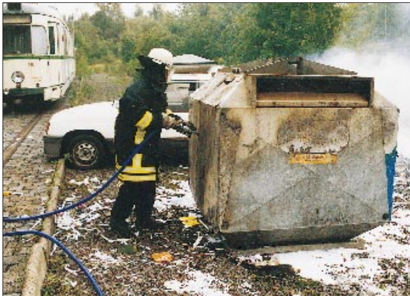
The homemade lance nozzle being used on a paper-recycling container at Wattenscheid.
