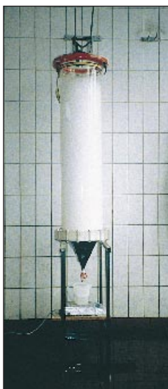
Above left and right: The clear acrylic tube used to collect samples of foam to measure aspiration and drainage time, and the actual sample-taking, with the author on the receiving end.
