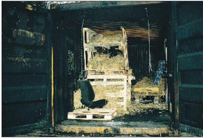
The 20-foot shipping container loaded with fuel and ready for ignition.
