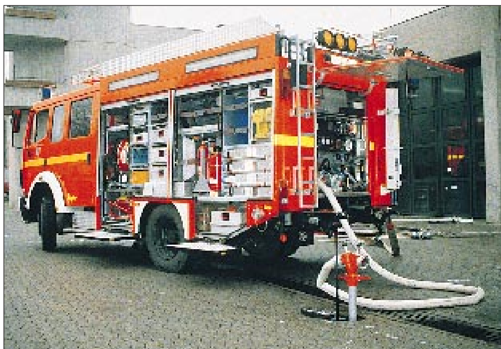
One of Ingolstadt's two new compressed-air foam pumpers, hooked up to a typical European below-grade hydrant.
